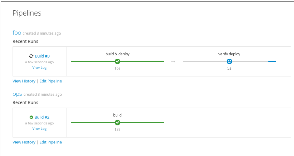
Figure 4-14. Cascading pipeline deployment using ImageChange triggers
